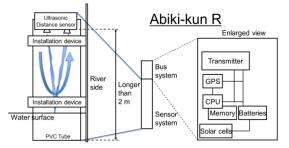
Figure 2: Ground sensor system with Abiki-kun R
